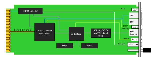
Figure 1: AMC227 Block Diagram
